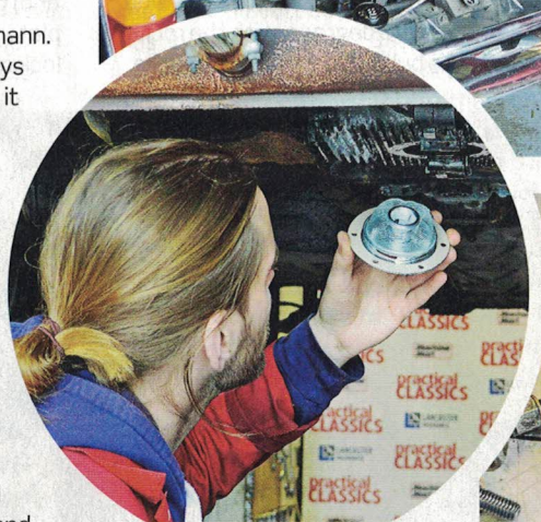
Replacement oil strainer and gasket went on easily.
